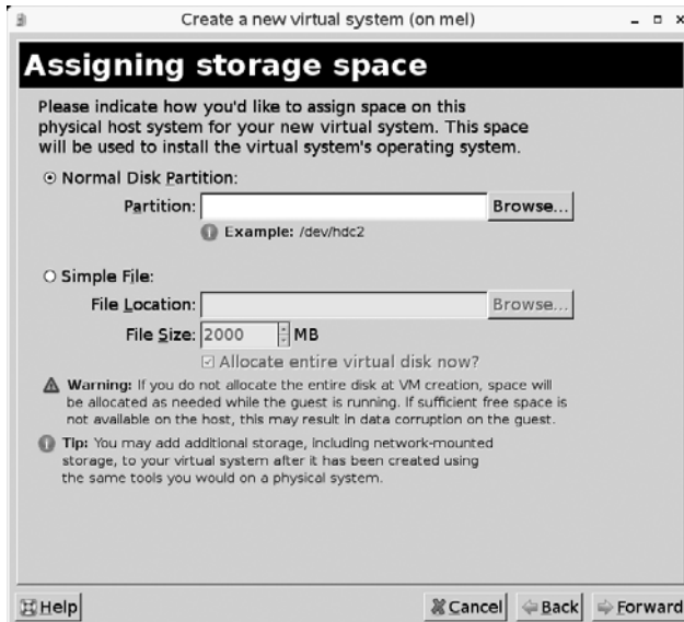
Figure 13-5. For best performance, use a partition or LVM logical volume as the storage backend.
